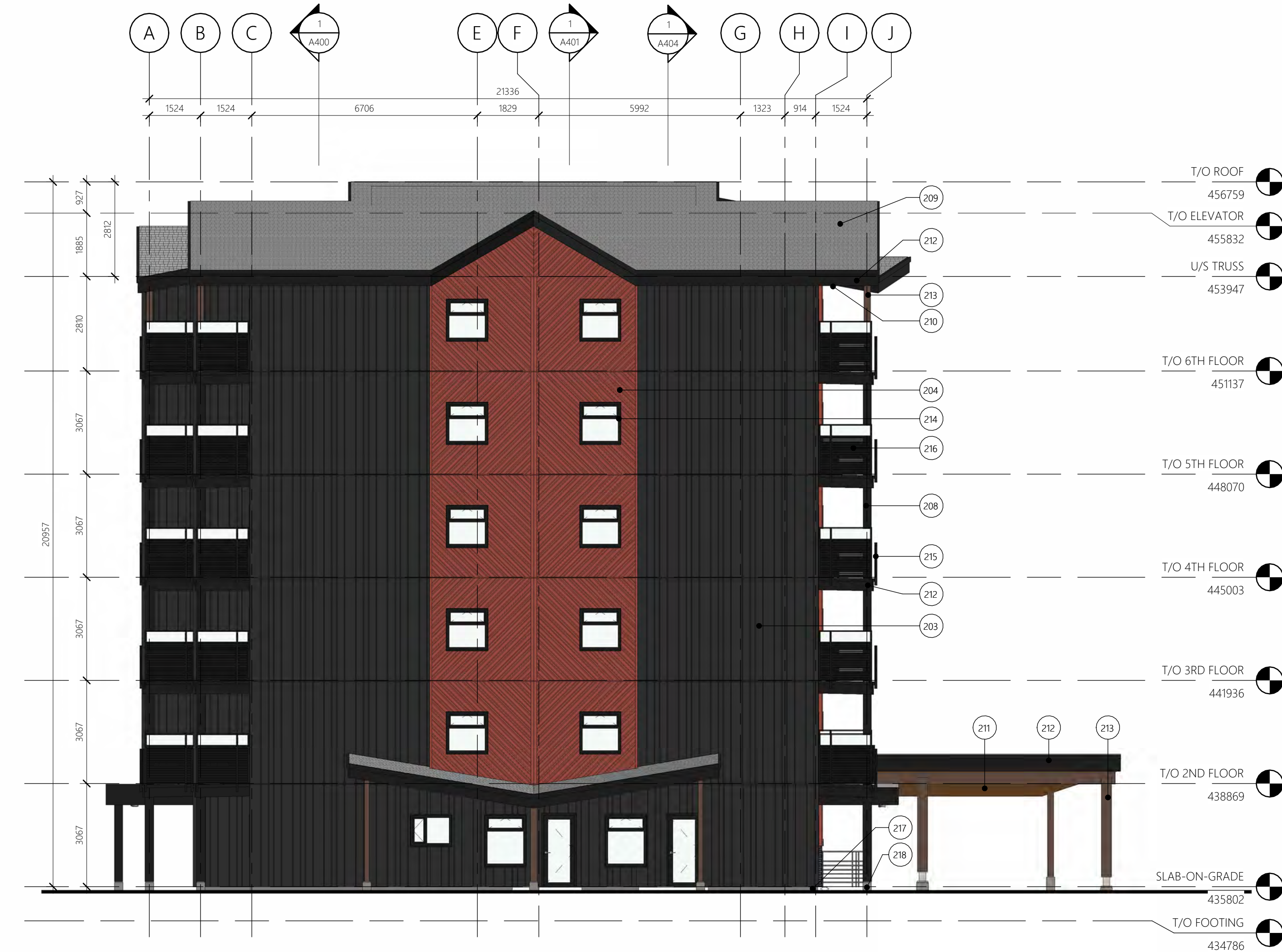
2 SOUTH ELEVATION - CLADDING
